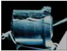
Cracked grommet during ozone test
