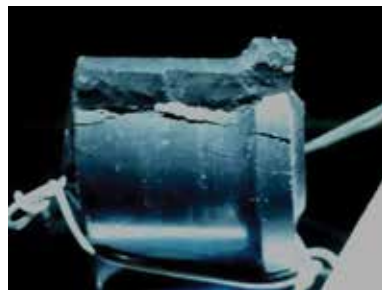
Cracked grommet during ozone test
