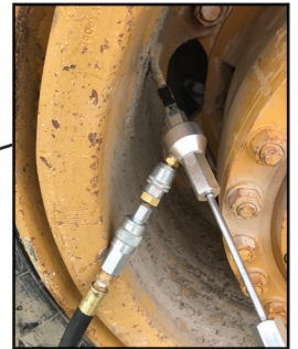
D. Large Bore Core Tool fastens to the valve for faster flow during inflation/deflation.
