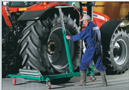
The Wheel Dolly for Agricultural and Earth Moving Machinery makes possible easy and safe mounting, demounting and handling of large wheels.
