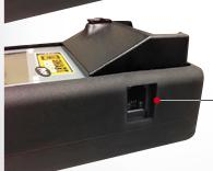
Later tools produced include the side port so it is only necessary to use the cable and the OBDII connector.
