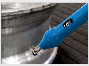
Ken-Tool®'s Valve Breaker quickly and easily removes valves.
