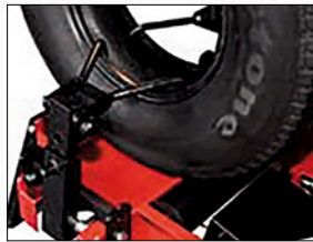
The Automatic Truck Tire Spreader in use.
