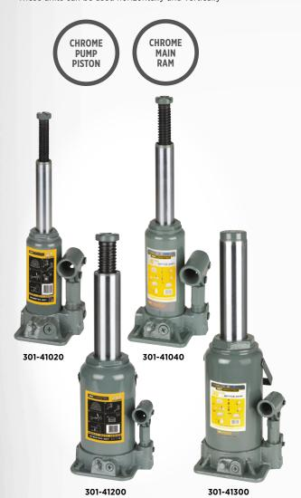
MIN. MAX. EXT. ASCOT NO. MFG. NO. CAPACITY HEIGHT SCREW HEIGHT G410200 301-41020 2-Ton 6-1/4" 11-3/4" 2" 301-41040 G410400 7-1/2" 14-1/2" 2" 4-Ton 301-41060 G410600 6-Ton 7-3/4" 14-3/4" 2" 301-41080 G410800 8-Ton 9" 18" 3-1/4" 301-41150 G411500 15-Ton 9-3/4" 19-1/4" 3-1/4" 301-41200 G412000 20-Ton 9-1/2" 18-1/2" 3-1/4" 301-41201 G412001 20-Ton Short 6-1/2" 11-1/4" 1-1/2"
