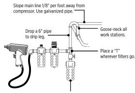
Place a drain trap at low points to remove water. Also utilize on main line at low points.
