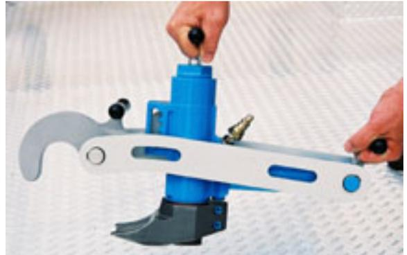
*Bead breaker with pin in lowest position.*
