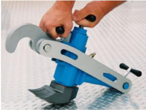
*Bead breaker with pin in highest position.*
