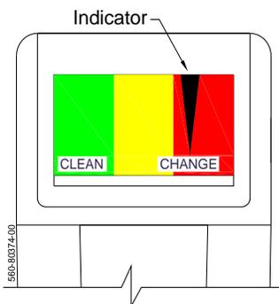
The condition of the Filter Element (mounted on rear of unit) can only be checked when shop air is connected to the unit and it is in the FILL TIRE mode of operation with Nitrogen being generated and filling the tank. It may be necessary to press the trigger on the fill wand to cause the tank filling. At all other times the Indicator will not be visible.
