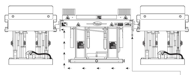
Air Hose Can Be Moved To Other Side If Necessary By Removing Bolt, Washer And Clip. Hose Is Wire Tied To Air Cylinder. Wire Tie Will Have To Be Cut And Reattached To Other Air Cylinder. Air Hose Must Be Located So That It Does Not Interfere With Swing Operation.
