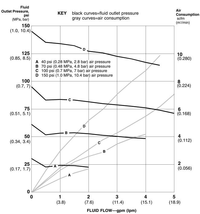
Test Fluid: No. 10 weight oil at 75° F (23.9° C)
