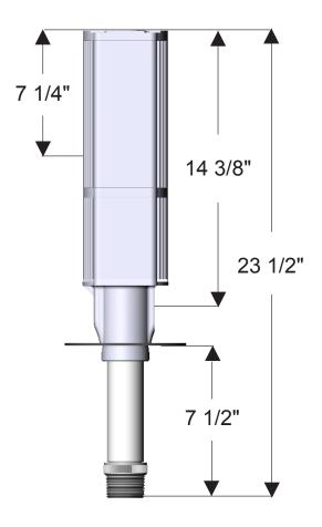
Flange Mount Pump Models 1130-017 & 1130-018 with Flange Mount Kit included with pump
