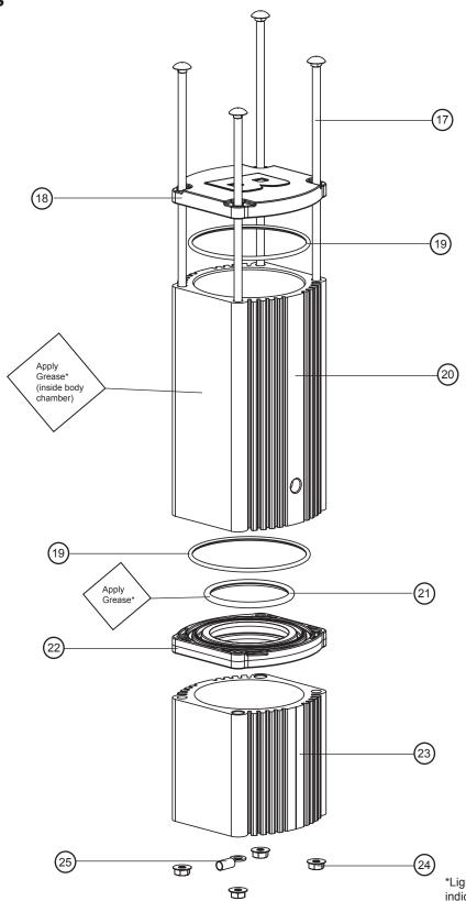
\*Lightly apply grease to surface indicated. Use Mobile Synthetic Lubricating Mobilith SHC PM.
