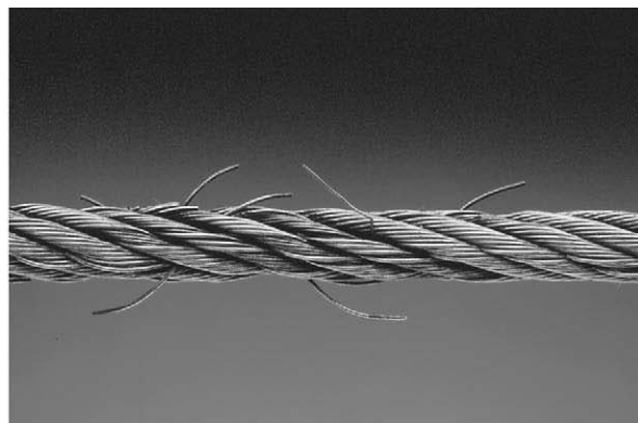
Cable With Broken Wires
