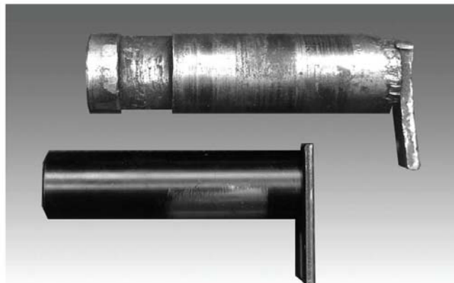
TOP PIN With Excessive Scoring and Wear
