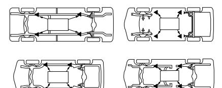
Lift Points Note: Pro9F 9000 lbs. Floor Plate Lift Refer to the manufacturer's specific vehicle lifting points. Some vehicles display these points on a label inside the right front door lock face or are identified by triangle shape marks on the vehicle's undercarriage, reference SAE J2184.
