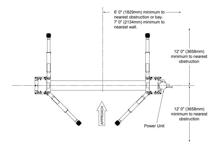
NOTE: Lift can be installed so power unit can column can be located on either side. However, to save operation steps it is recommended that it is placed on passenger side of lift.
