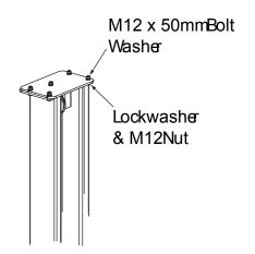
**STEP 5**: Install the top plate onto the top of the columns. **NOTE: 1" = 25.4mm**
