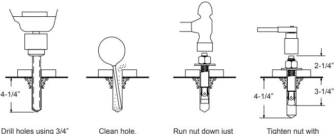
carbide tipped masonary drill bit per ANSI standard B94.12.1977
