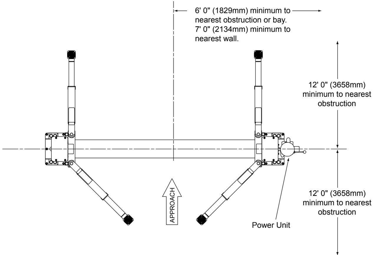
**NOTE: Lift can be installed so power unit can column can be located on either side. However, to save operation steps it is recommended that it is placed on passenger side of lift.**
