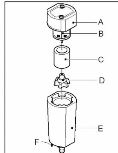
**Note:** A periodic check of the automatic drains is necessary to ensure maximum membrane life. To verify float is functioning correctly, open the filter bowl by turning one quarter turn counter-clockwise. Inspect for water or oil, an inactive float will be submerged, an active float will not. If float is found to be inactive follow clean automatic drain procedure or if necessary replace with part number 026-80386-00.
