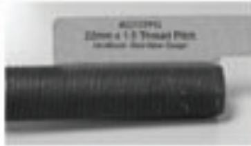
Gauge with New Stud
