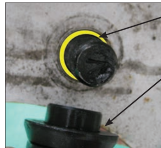
Void (Highlighted in Green) between stud and hole.
