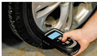
The Bartec Tech 500 All-In-One TPMS Service Tool in use.
